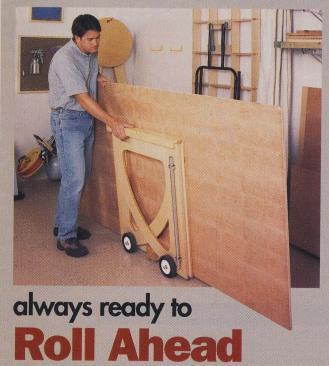
When you need to move a sheet of plywood more than just a couple feet, fold the shuttle into a two-wheeled cart. This is excellent for taking sheet goods through gates or doorways, or even moving it from your truck to your lumber storage rack.
